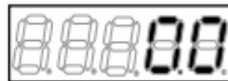
"0.0" Hz displayed as output frequency when the inverter is stopped in [V/f]
